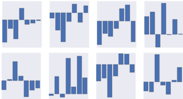
Figure 3: Convolution weights learned by the CNN on the step count time series of the UPTAKE dataset. Each graph shows the 7 learned weights for each of the nodes in the first convolutional layer for step counts.
